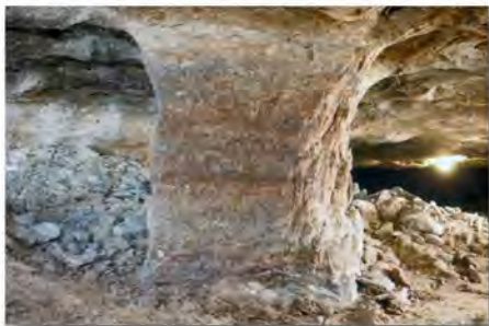
Underground Potash Pillar
